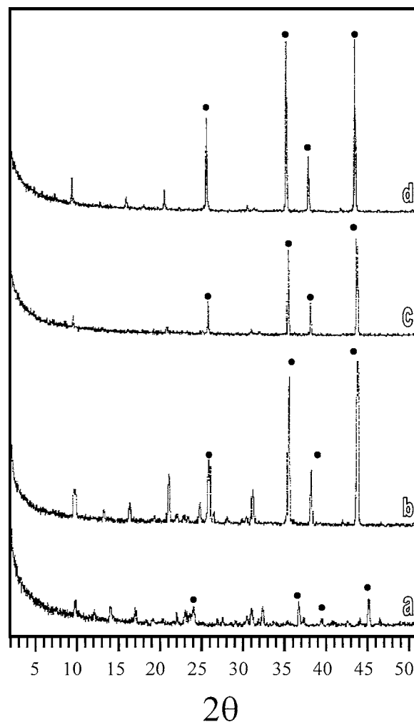
Figure 1 XRD patterns of aluminophosphate molecular sieve films. (a) as-synthesized AlPO 4 -14 film on porous alumina tube, (b) as-synthesized CoAPO-44 film on dense alumina plate, (c) calcined CoAPO-44 film on dense alumina plate, (d) as-synthesized ZnAPO-34 film on dense alumina plate.
